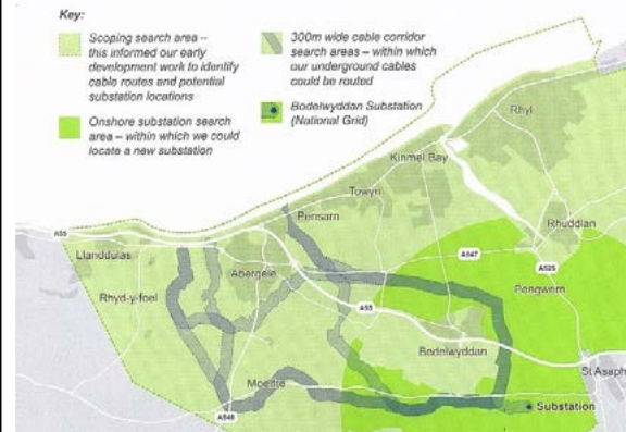
Possible routes for the underground cabling
