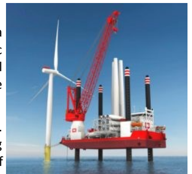
"Jack-up" vessel installing a turbine. Worth looking up on youtube to learn more!
