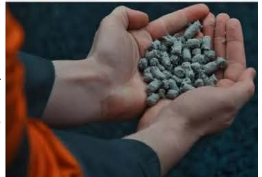
A 1.4-mile stretch of road between Cardigan and Aberystwyth has been re-paved using 107,000 recycled disposable nappies. Fibre from the nappies is added to the bitumen that glues together asphalt road surfaces. (images: Pura)
