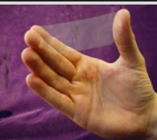
Coverglass: from 50 to 500 microns thick for satellite solar cells as below
