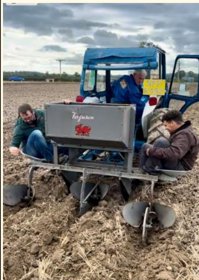
A 1950s Ferguson potato planter. The lads drop a seed potato down the chute in time with a bell.
